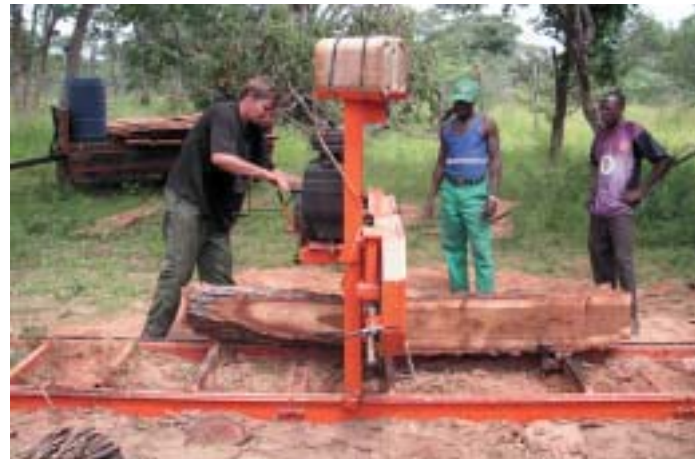
Left: logs dragged to the nearest processing point; right: logs sawn in planks with a mobile saw mill.
